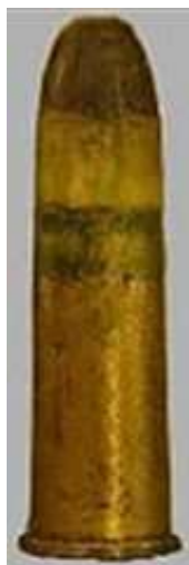
The first type 7.5mm Swedish cartridge. Black powder & paper patched bullet.
