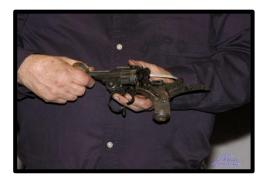
double action only (DAO) break-top that copied features of several different European and American (primarily Smith & Wesson) designs. It is chambered in a unique 9mm caliber. It can be disassembled without any tools!
