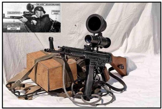
Another unusual (for the time) accessory was the Zielgerat 1229 "Vampir" night vision system (*above*) introduced in February 1945. Consisting of an Infrared light (illuminator), optics, and a large (~30 lbs) battery pack, the Vampir was one of the very first night vision device deployed in combat.
