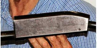
L: Ed Costello shows his Winchester Model 59 lightweight field shotgun. R: Model 59 Cracked receiver – note horizontal crack running the length of the receiver, a typical problem when high brass hunting loads were used.
