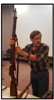
more robust barrel band, and the ability to mount the sling either on the side or underneath. This example was made by Sako and the barrel has a .311 bore.
