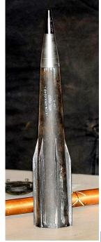
Left: The dummy long rod penetrating round with discarding sabot anti-tank round. Note the long rod on the table top.
