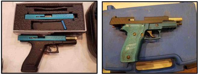
Left: Glock with conversion barrel and slide. Right: Sig converted to operate with non-lethal rounds
