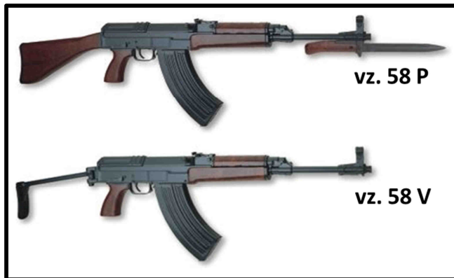
There are three variants of the vz.58 - the fixed stock infantry rifle vz.58 P (top left), the side folding stock paratrooper rifle (bottom left), and the infrared night sight-equipped vz.58 Pi (right)
