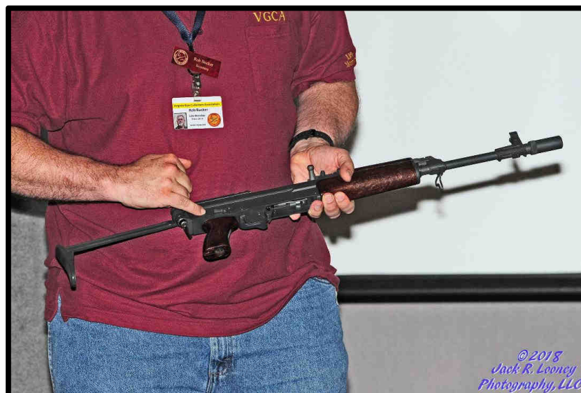
Rob explains the selector lever on his semi-automatic vz.58 V. Note the permanently attached muzzle device to ensure that the original military barrel is over 16 inches long, as required by the NFA.
