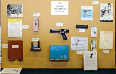
The Second Place Award went to **Ernie Lyles** for his display on *The Dardick Magazine-Fed Revolver*. The revolver used triangular cartridges called "trounds" which were fed from a magazine into a cylinder and then revolved into place for firing. Also included was rare documentation related to the design, development and patenting of the gun, as well as manuals and sales literature.
