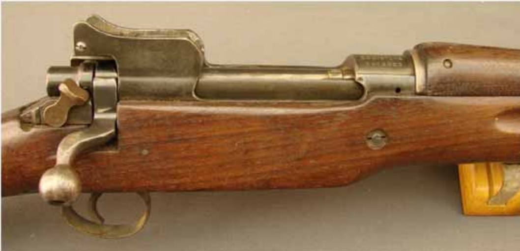
M1917 Right side of action showing deep wood around magazine, crooked bolt handle, safety, and "ears" protecting the rear sight. Photo: www.joesalter.com
