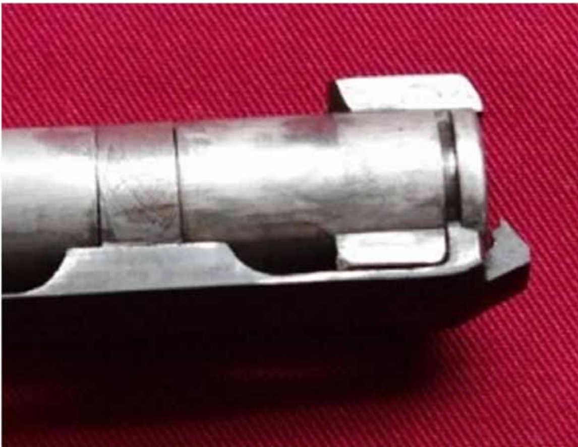
Winchester P-14 Mk I bolt. Note the locking lug. Photo courtesy of Barry Bromley – www.classicfirearms.be
