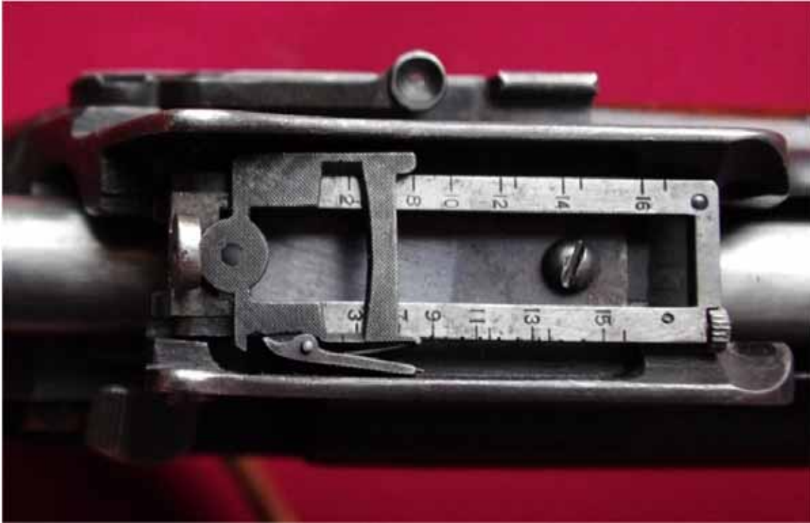
P-14 Mk I W (F) Winchester top showing Action & Fine Adjustable Rear Sight. Note the knob at the top of the leaf for fine adjustments and the archaic rear volley sight on the left side. Photo courtesy of Barry Bromley – www.classicfirearms.be
