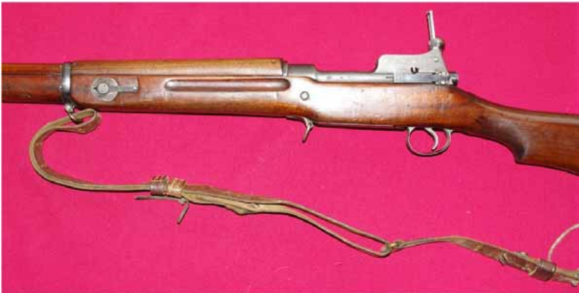
P-14 Mk I W (F) Winchester Left side with rear sight leaf raised. It still retains its front and rear volley sights. Neither the sling nor the sling swivel in front of the magazine floor plate are regulation and may have been added for use in target matches. Photo courtesy of Barry Bromley – www.classicfirearms.be
