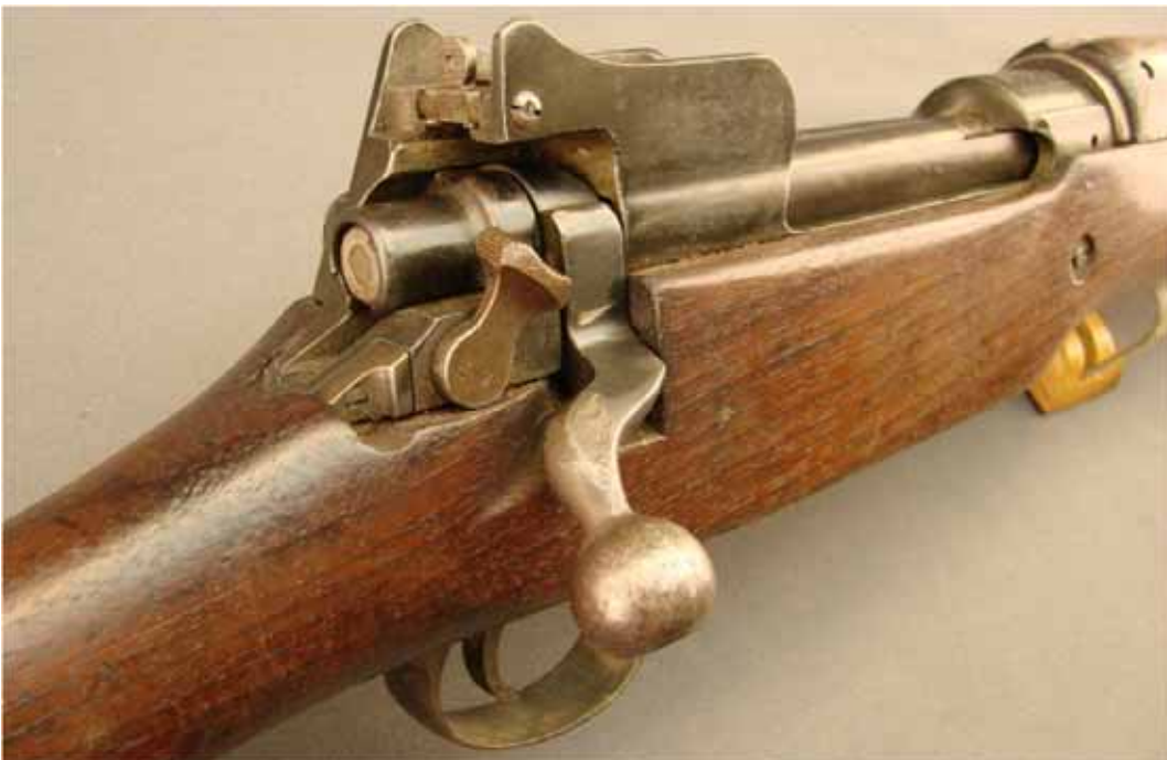
M-1917 another view of crooked bolt handle, safety, rear sight and "ears" protecting the rear sight. Photo: www.joesalter.com
