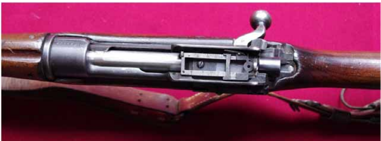
Pattern 1914 Mk I W (F) Winchester top showing Action & Fine Adjustable Sight.
