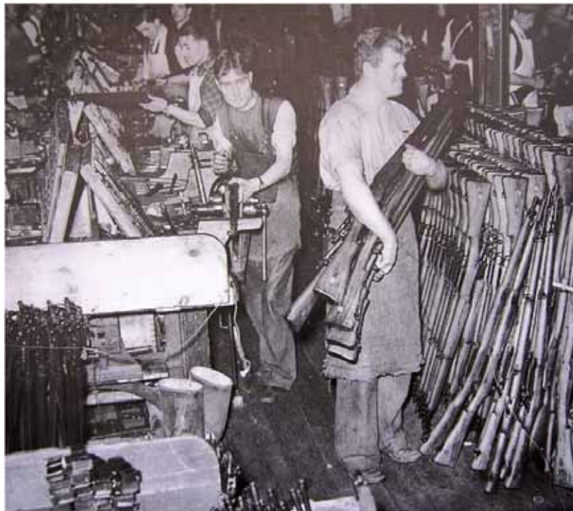
Weedon Repair Depot Refurbishing P-14s (Public Domain)
