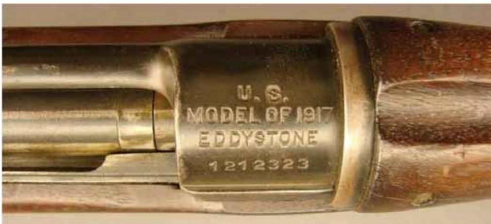
M-1917 Eddystone manufacturer prime markings on top of receiver ring. Photo: www.joesalter.com
