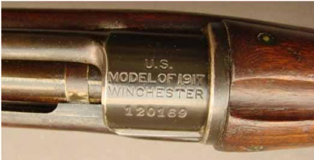
M1917 Winchester manufacturer primed markings on top of receiver ring. Photo: www.joesalter.com
