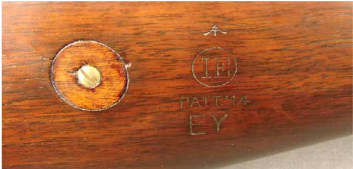
P-14 with British markings on butt stock. The letters "IE" in the circle identify it as an Eddystone. The (apparently hand-applied) 'EY' marking donates reclassification to 'Emergency Use' only [Appx E, page 216 – Major E G B Reynolds, 'The Lee Enfield Rifle' pub 1960] Photo: www.joesalter.com
