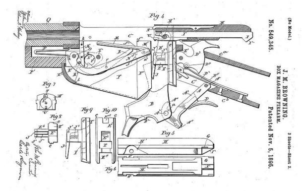
Fig. 5 – Drawing 2 from Browning Patent 549,345, Nov. 5, 1895 showing the action open with the lever down. U.S. Patent Office.
