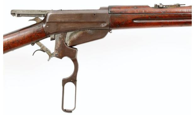
Fig. 4 – Close up of the open action with lever down of U.S. marked Winchester Model 1895, S/N 17893. Photo Tim Prince, College Hill Arsenal.
