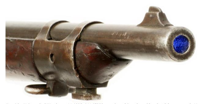
Fig. 16 – U.S. marked Winchester M-1895, S/N 17893, muzzle and front barrel band with bayonet stud. Note the ramp front sight with pinned blade. Photo: Tim Prince, College Hill Arsenal.
