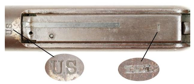
Fig. 13 – U.S. marked Winchester M-1895, S/N 17893. Note **U.S.** stamp on the receiver and the **KSM** inspector initials. Photo: Tim Prince, College Hill Arsenal.
