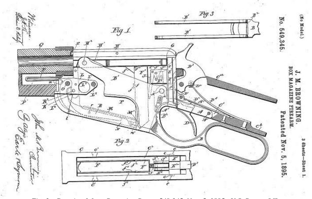
Fig. 3 – Drawing 1 from Browning Patent 549,345, Nov. 5, 1895. U.S. Patent Office.
