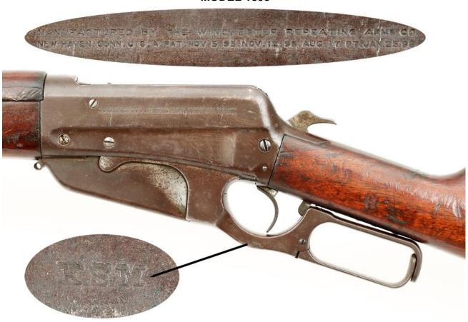
Fig. 12 – U.S. marked Winchester M-1895, S/N 17893, left side. Note the manufacturer's stamp on the receiver and the inspector's initials, **KSM** on the lever. Photo: Tim Prince, College Hill Arsenal.
