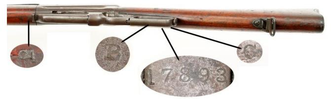
Fig. 15 – U.S. marked Winchester M-1895, S/N 17893, bottom view. Note the location of the sub-inspector stamps. The serial number is located on the lower tang underneath the closed lever. Photo: Tim Prince, College Hill Arsenal.
