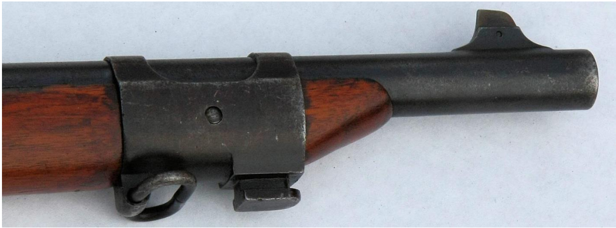
Fig 9 – Detail of front barrel band, front sight and bayonet lug. Photo – Bill Chronister
