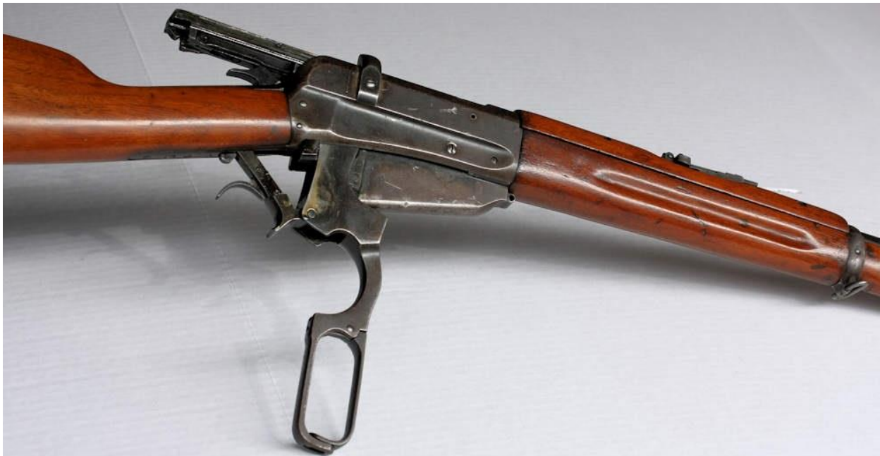
Fig 6 – Winchester Russian Model 1895 receiver, action open. Photo – Bill Chronister
