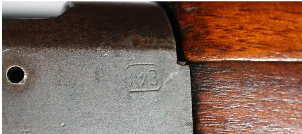
Fig 16 – Russian inspection stamp on the right side of the receiver. Photo – Bill Chronister
