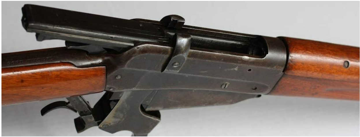
Fig 11 – Winchester Russian Model 1895 receiver, action open showing the 2-piece loading bridge with guides for stripper clips. Photo – Bill Chronister
