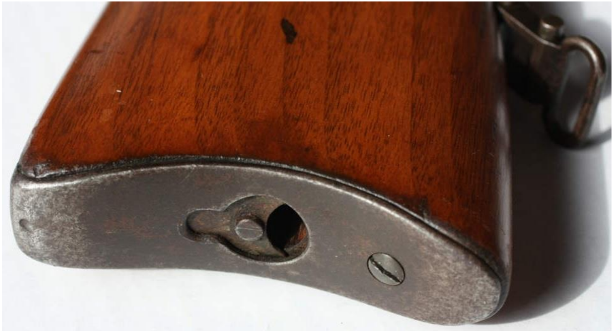
Fig 7 – Buttstock with sliding trapdoor to compartment for cleaning kit and disassembly tool. Photo – Bill Chronister
