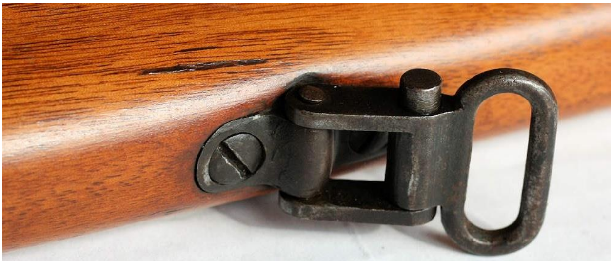
Fig 8 – Detail of quick detach sling swivel on the buttstock. Photo – Bill Chronister
