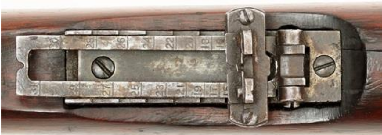
Fig 10 – Winchester Russian Model 1895 rear sight. Photo – Tim Prince, College Hill Arsenal
