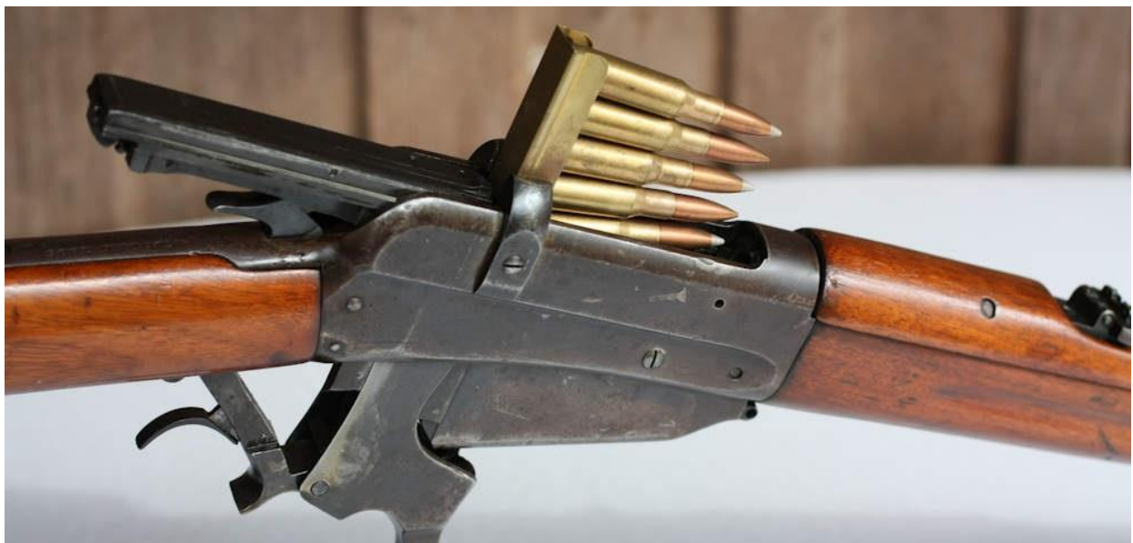
Fig 12 – Winchester Russian Model 1895 receiver, action open 2-piece showing stripper clip with ammunition inserted into loading bridge. Photo – Bill Chronister
