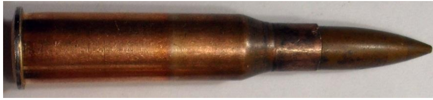
Fig. 4 – Russian 7.62x54mmR Cartridge. Photo Public Domain.
