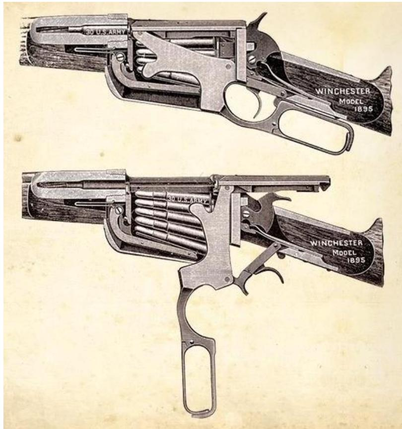
*Fig. 6 – Cutaway drawing of action of Winchester Model 1895 from Winchester 1899 sales catalog. Public Domain.*
