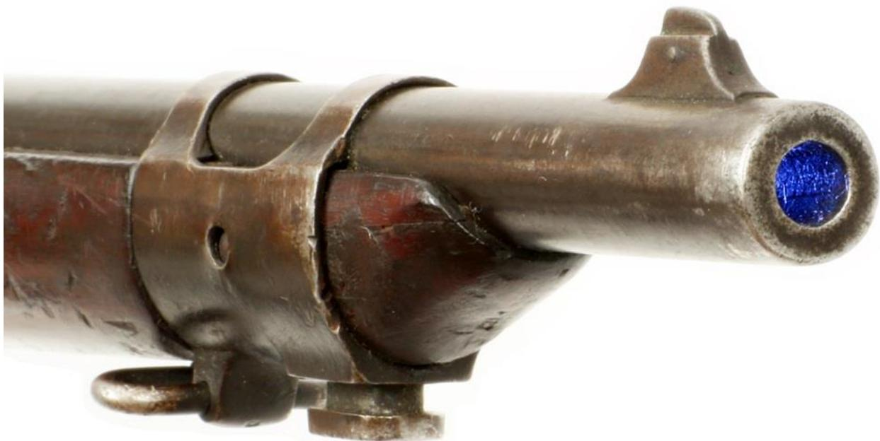
*Fig. 16 – U.S. marked Winchester M-1895, S/N 17893, muzzle and front barrel band with bayonet stud. Note the ramp front sight with pinned blade. Photo: Tim Prince, College Hill Arsenal.*
