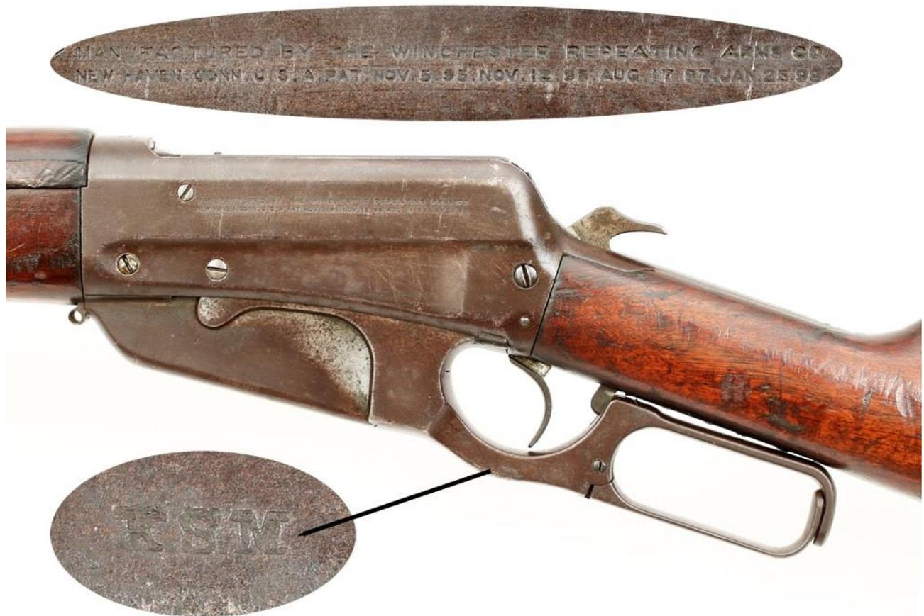
*Fig. 12 – U.S. marked Winchester M-1895, S/N 17893, left side. Note the manufacturer's stamp on the receiver and the inspector's initials, **KSM** on the lever. Photo: Tim Prince, College Hill Arsenal.*
