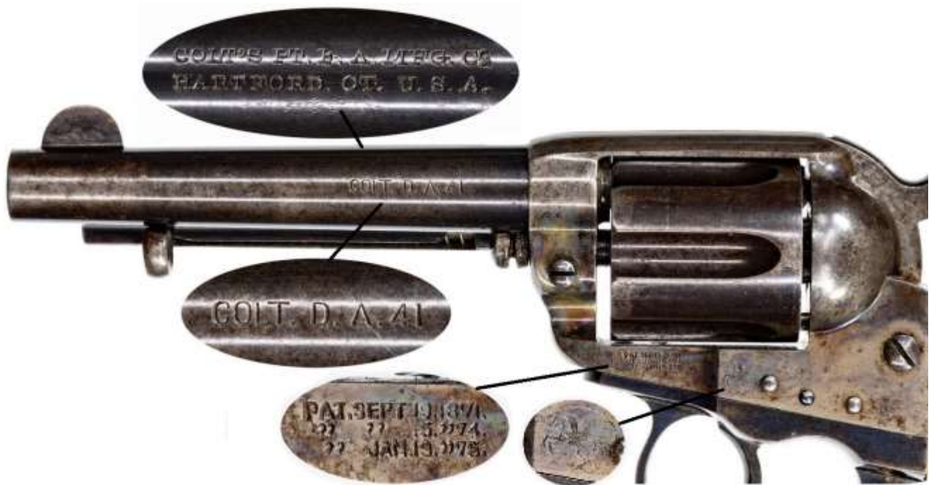
Colt Model 1877 "Thunderer" .41 caliber, serial number 106123 produced in 1897. Blued barrel and cylinder and color case hardened frame. Mother of Pearl grips, 4 ½" barrel and rod ejector. Note the Colt address on top of the barrel, the roll marked caliber on the side of the barrel, and on the frame the three line Colt patent mark and ramphant colt. Photo by Tim Prince, College Hill Arsenal.
