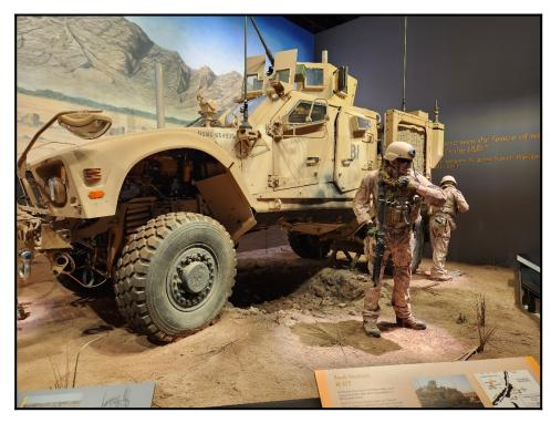
Shown here is a Mine-Resistant Ambush Protected (MRAP) All-Terrain Vehicle (M-ATV) (left). Intended to replace M1114 HMMWVs (Humvee), it was designed to provide the same levels of protection as the larger and heavier previous MRAPs, but with improved mobility to handle the poor roads and difficult terrain of Afghanistan. This M-ATV still has the battle damage from when it hit an improvised explosive device (IED) while delivering supplies in Helmand Province, Afghanistan.
