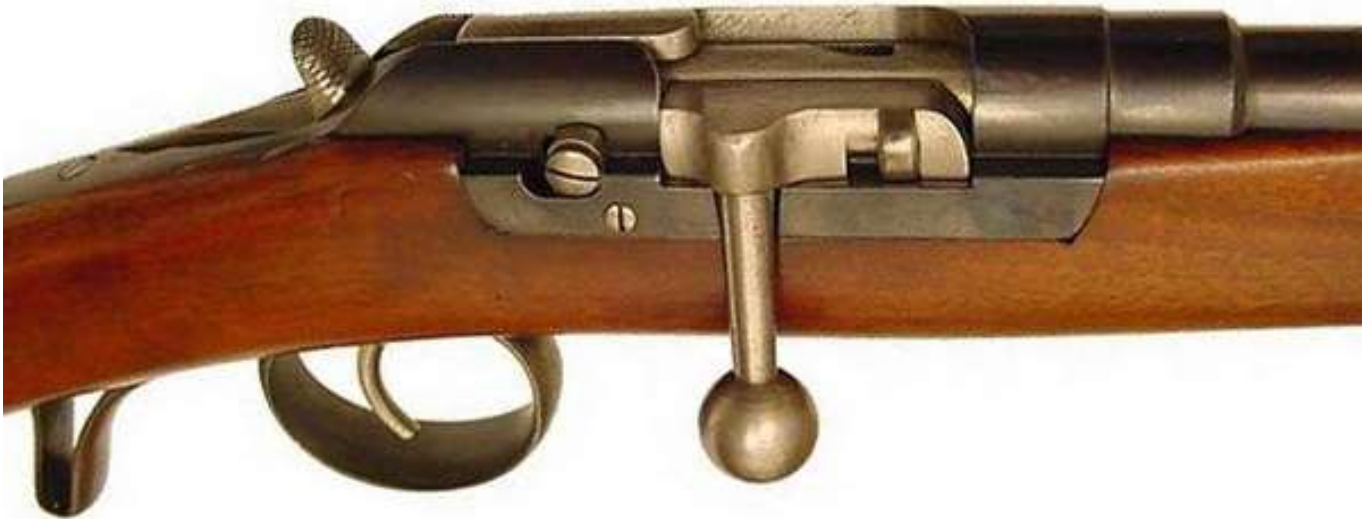
Fruwirth M1872 carbine with bolt closed. Note magazine cut-off switch in front of bolt handle that prevents the cartridge elevator from lowering to pick up cartridge fed from the tubular magazine. Photo – Weaponland
