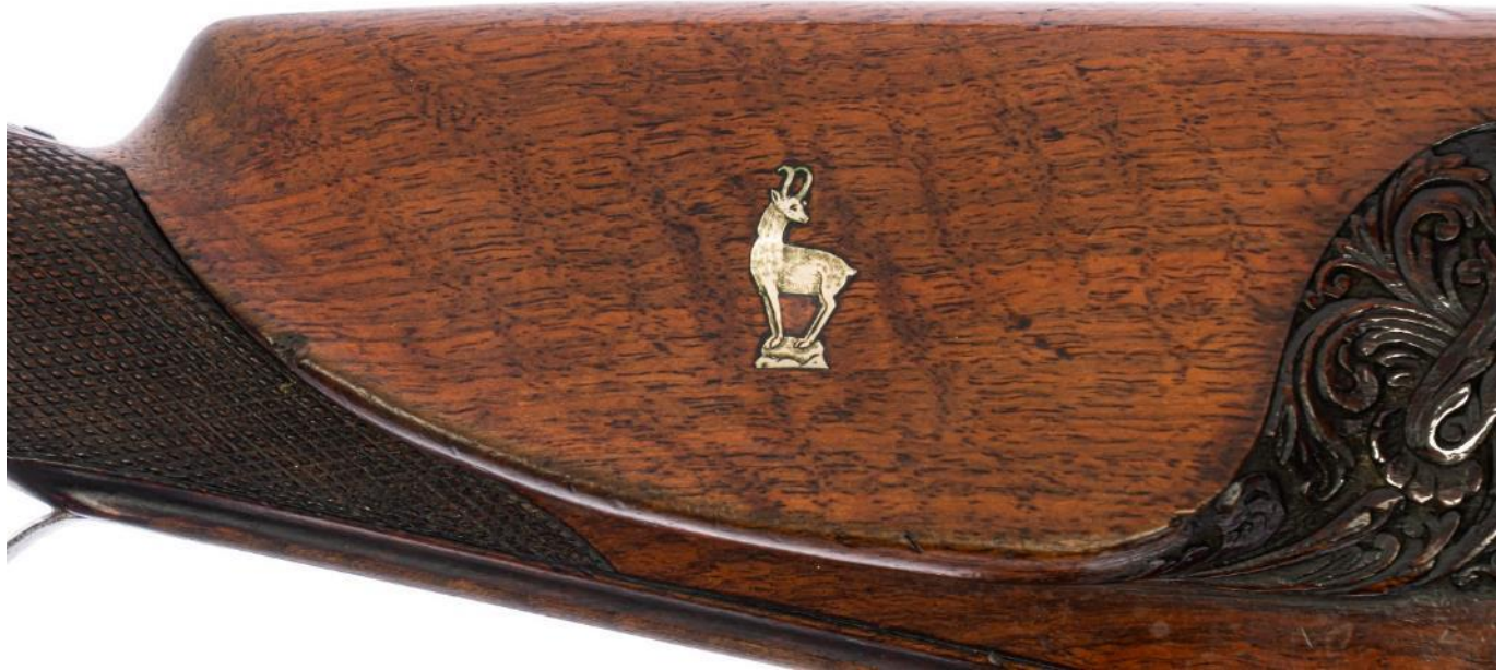
Leithner's trademark, a gold chamois is inlaid into the cheekpiece of the stock.
