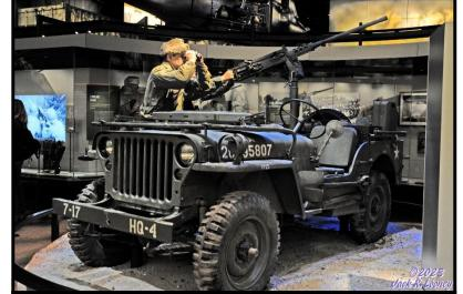
Two American G.I. classics (*left*) – an M2 50 caliber machinegun (another John Moses design) mounted on ½ Ton 4x4 Willys Jeep. The Jeep was developed right before the U.S. entered WWII and almost 650,000 were produced during the war. Replacing horses and mules in U.S.
