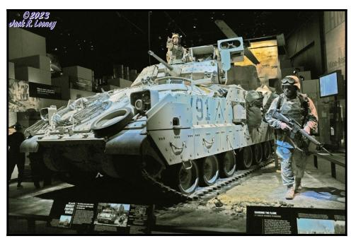
Named for General Omar Bradley, the Bradley Fighting Vehicle (left) mounts a 25mm M242 Bushmaster chain gun, two BGM-71 TOW (Tube-launched, Optically tracked, Wireguided) anti-tank missiles, and an M240 coaxial machinegun. The "upside down V" on the side of the hull was an Allied identification symbol used during Operation Desert Storm in 1991, much like the "Z" seen currently painted on Russian vehicles fighting in Ukraine.
