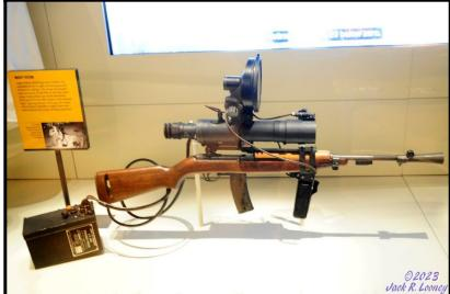
The M3 with M2 sniper scope (*left*) was an early attempt at creating a night vision capability. Deployed right the end of WWII (replacing the first T3 variants), it consisted on an M2 select-fire carbine with an infrared spotlight (on top), television type cathode ray scope to "see" the target, and associated battery pack carried in a backpack. Ungainly and heavy, it had a range of approximately 100-120 yards. The M3 with the M2 sniper scope saw service during the Korean War and into Vietnam.
