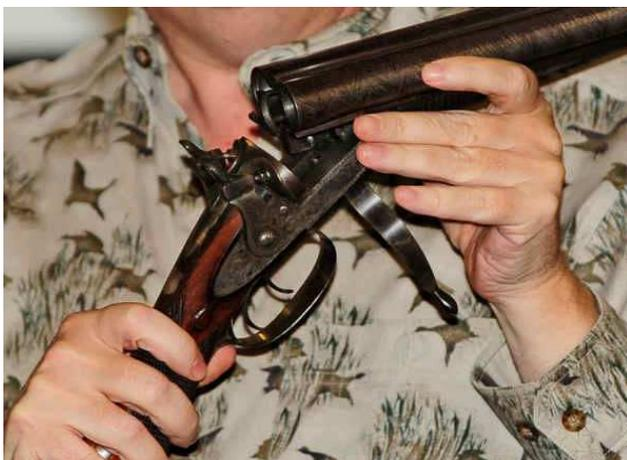
L: Receiver and lock area of Charlie Rathell's side-by-side percussion underlever, hammer shotgun that was converted to centerfire.
