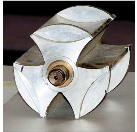
**R-top:** Prototype of an experimental 25mm Naval gun that was never developed shows the unique Dardick cylinder design features.
