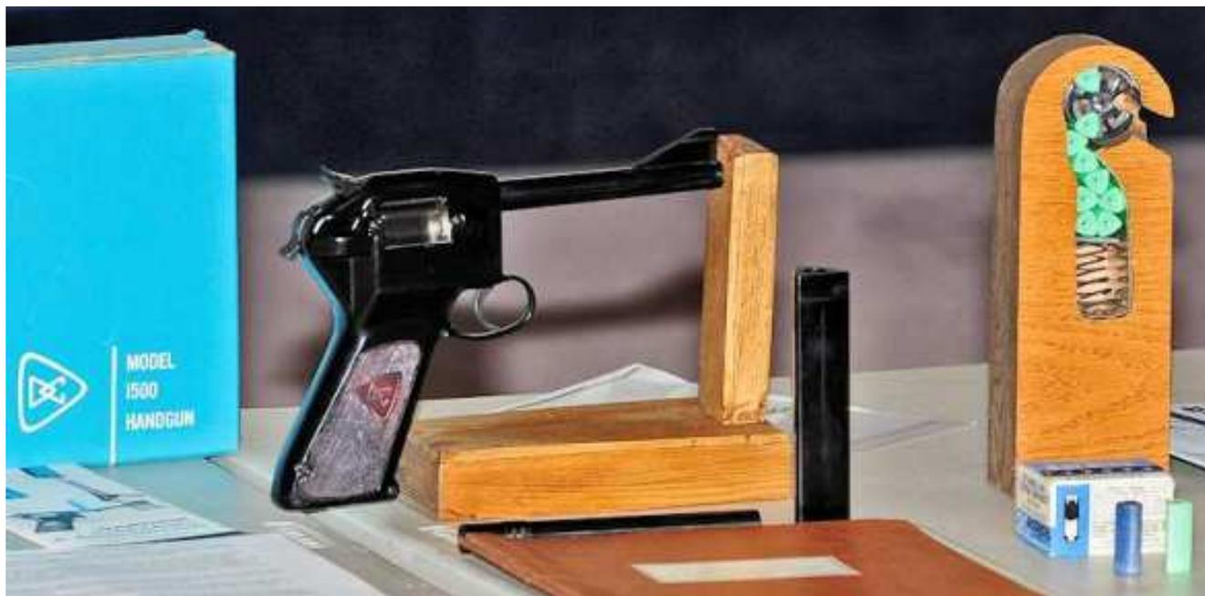
**L:** The Model 1500 Dardick Revolver with a wooden model of the magazine (right) to demonstrate the loading, feeding, and ejection of trounds. Below are sample trounds.
