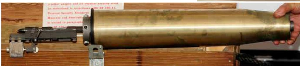
↙ 90mm tank gun sub-caliber training device
