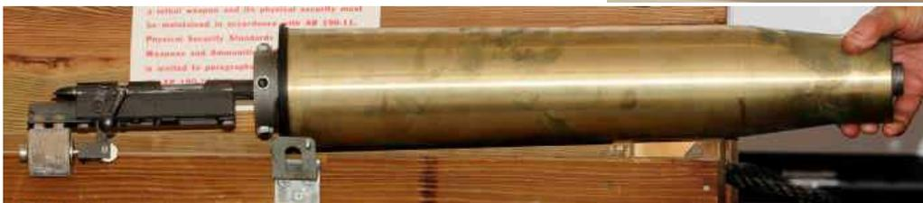
↙ 90mm tank gun sub-caliber training device
