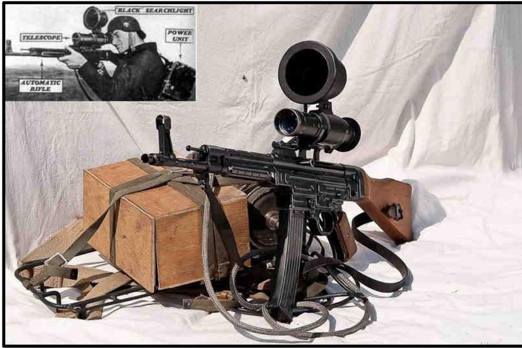
Another unusual (for the time) accessory was the Zielgerät 1229 “Vampir” night vision system (*above*) introduced in February 1945. Consisting of an Infrared light (illuminator), optics, and a large (~30 lbs) battery pack, the Vampir was one of the very first night vision device deployed in combat.
