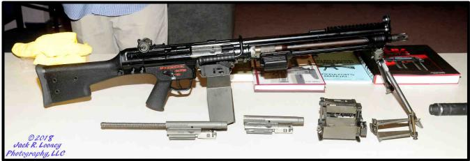
Here is another example of H&K engineering excellence! This belt-fed, bipod-equipped piece of hardware is an HK 23e machine gun with conversion kits for the HK 11e and HK 21e
