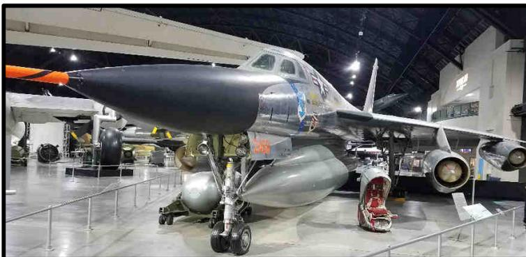
One of the sleekest planes ever fielded by the USAF was the B-58 “Hustler” (*left*). This 1960s bomber was designed to deliver nuclear bombs at Mach 2, but was expensive to maintain and quickly outmoded by advanced Soviet Surface-to-Air missiles.
