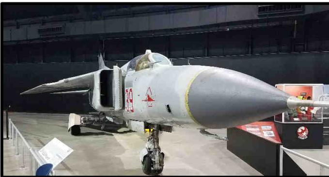
MiG-23 “Flogger” (*left*). This high-speed interceptor featured variable geometry “swing” wings and was one of the first Soviet fighters to have a radar that could look down and distinguish targets from ground clutter. It is a little known fact that in the 1970s and ‘80s the USAF operated a squadron of MiGs (known as the “Red Eagles”) from a secret base in the Nevada desert to provide familiarity training to U.S. pilots. This MiG was part of that program.
