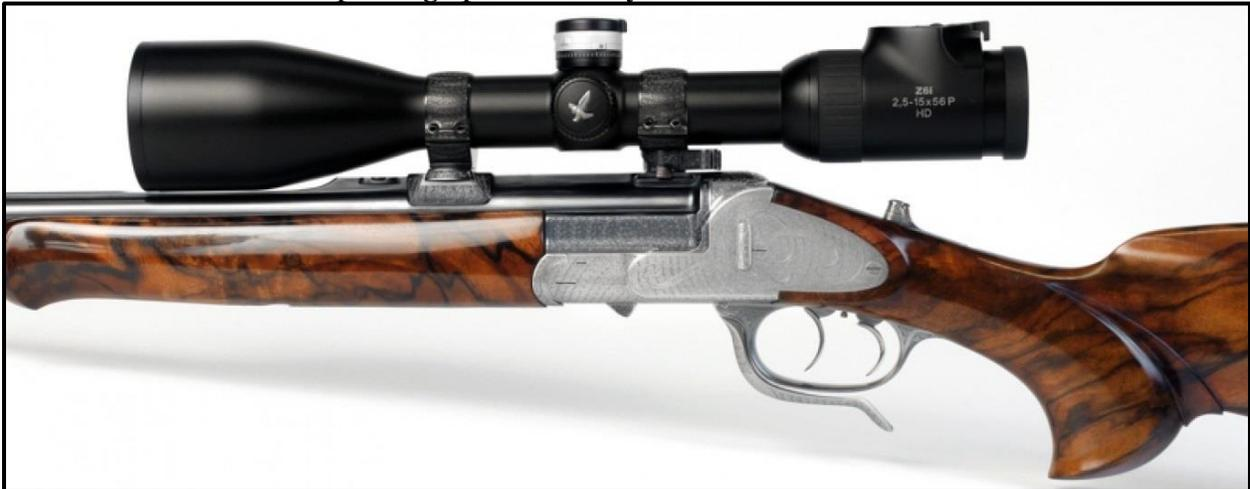
It has adjustable double set triggers and selection between the barrels is made with a sliding lever on the left hand side of the action. Fine hand scroll and floral engraving and ornaments adorn the action, sights, mounts, trigger guard and the underlever.
