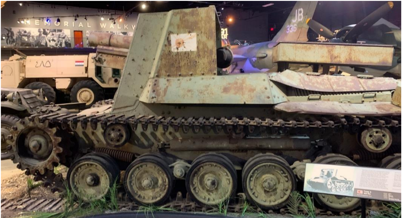
Extremely rare Japanese Type 4 Ho-Ro Self-Propelled Howitzer with a 150mm gun. Only 12 Ho-Ros were produced. This one was captured in Luzon, Philippines and is the only Ho-Ro still in existence..
