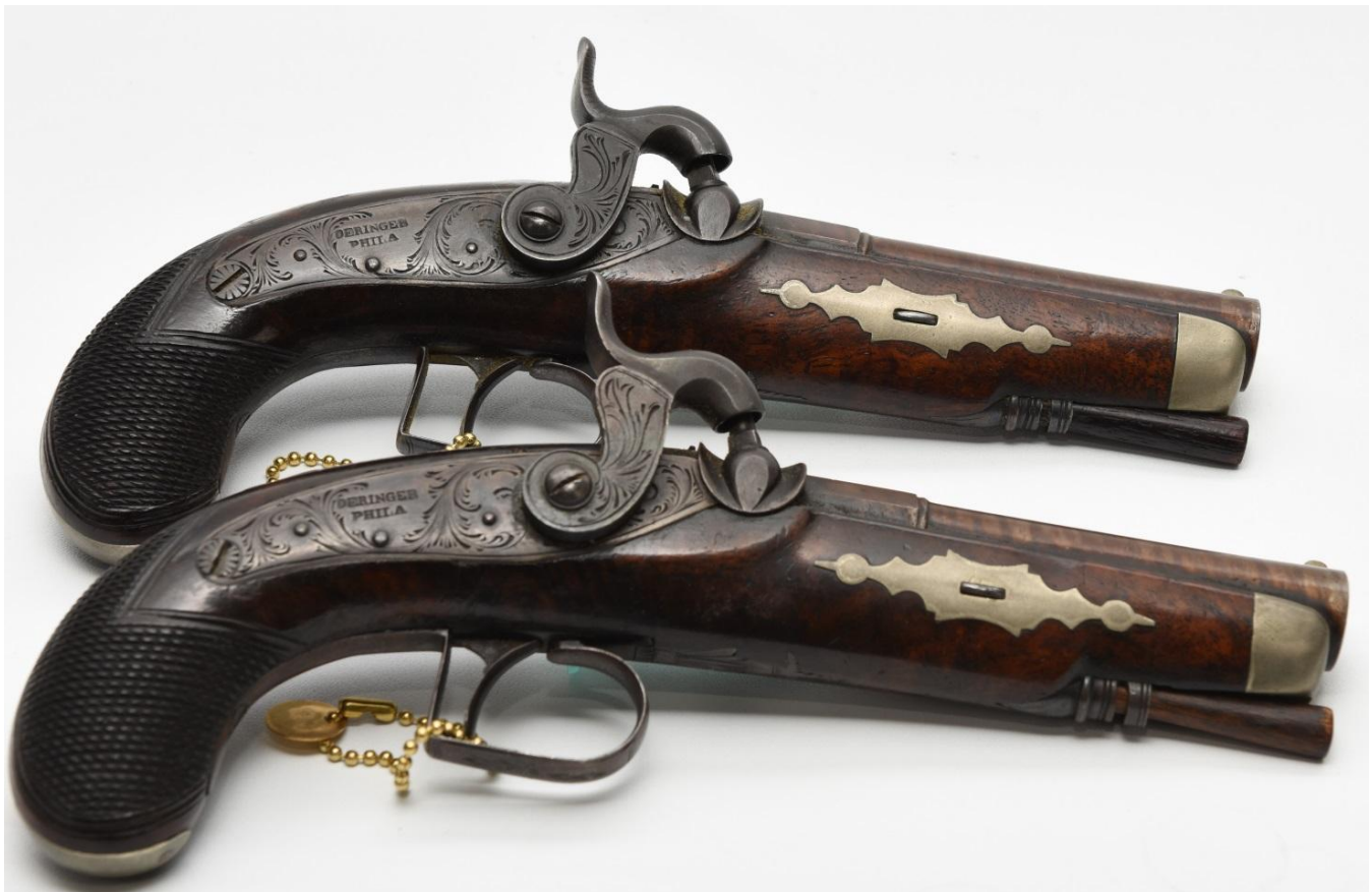
The Talcott 2 nd generation “Deringer” circa 1828-1830. Note the back action locks and the shorter part-round, part octagonal barrels.
