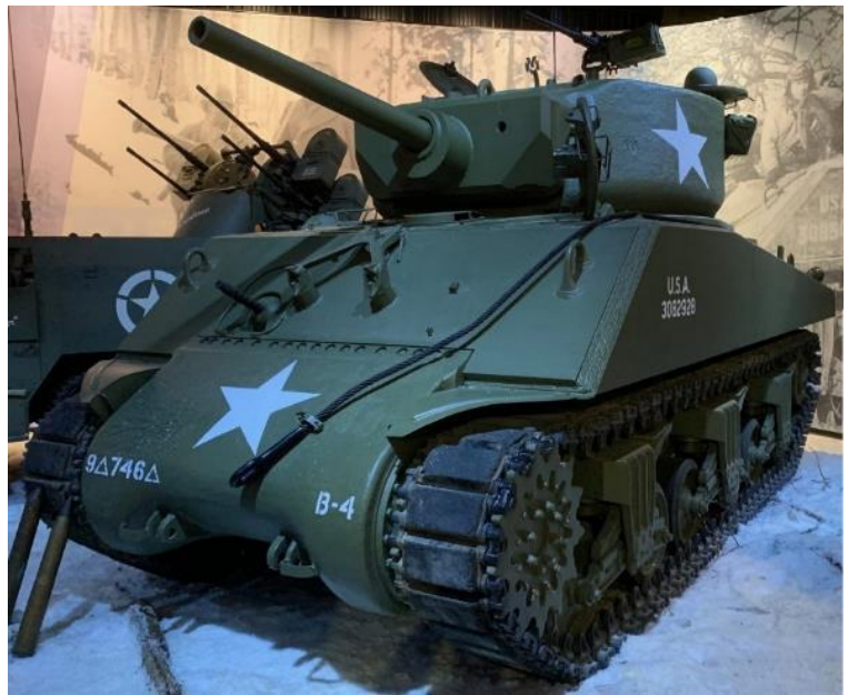
Left – US M8 75mm Self Propelled Howitzer. Right – US M4A3E2 Sherman “Jumbo” Heavy Assault Tank, a rare up-armored version of the M4 Sherman. One of the first Jumbos produced, it still shows battle damage on the front transmission housing. A Sherman Jumbo was the first tank to reach the besieged 101 st Airborne Division in Bastogne during the Battle of the Bulge.
