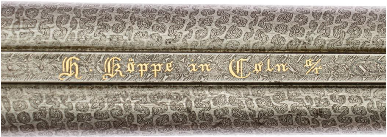
Heinrich Köppe's name, inlaid in gold on the rib. Note the spiral patterns on the barrels and the engraving on the rib between the barrels.
