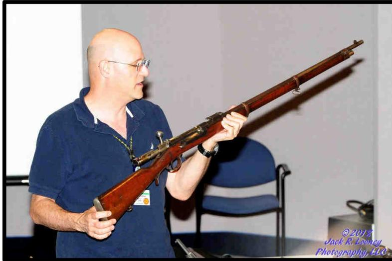
Member 3 (*above*) presented a Portuguese Model 1886/98 Kropatschek rifle. Made in Austria by Steyr, the M1886 features an 8-round tubular magazine under the barrel (similar to the German Model 1871/84) and was originally chambered in the 8x60mm blackpowder round. This particular example was converted in 1898 to use the smokeless powder 8x56r with an updated rear sight to match the higher-velocity round.
