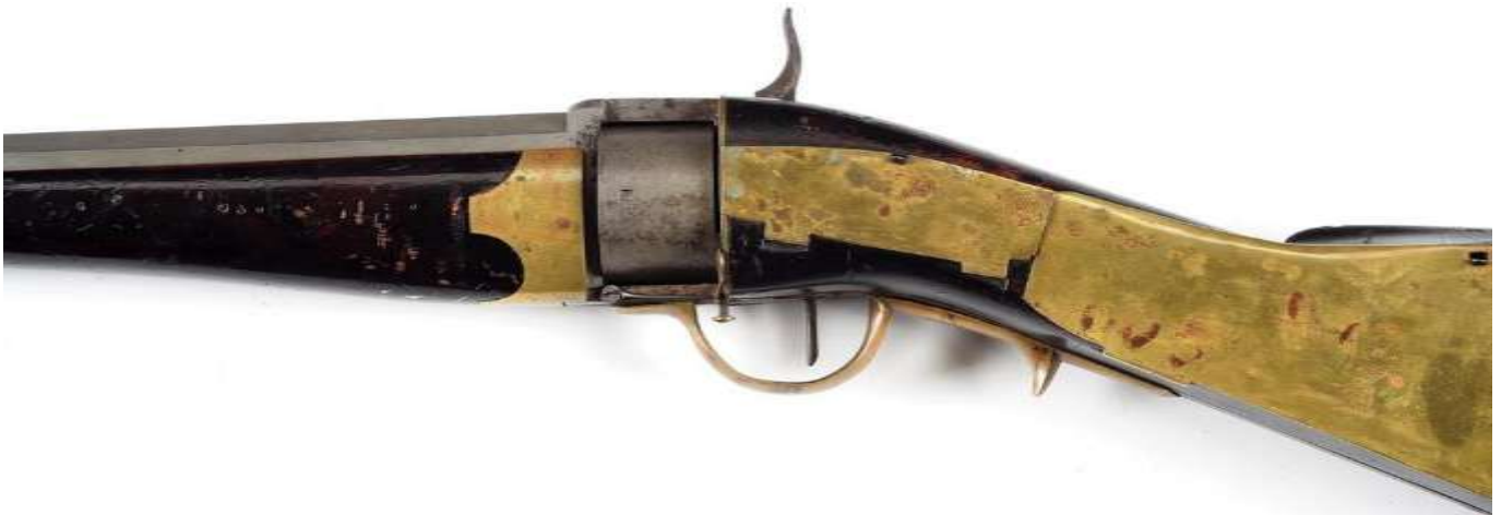
Benjamin Parkinson Revolving Rifle. Note the brass doors on the stock covering the "magazine" chamber and mechanism. Photo courtesy of Morphy Auctions, Denver, PA.
