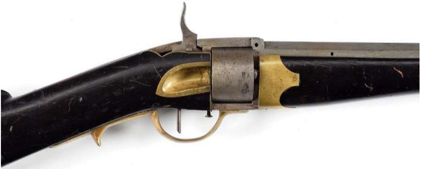
Benjamin Parkinson Revolving Rifle. Right side showing the hammer and steel cylinder. The brass groove above the trigger is presumably for loading/ejection of spent cartridges. Photo courtesy of Morphy Auctions, Denver, PA.
