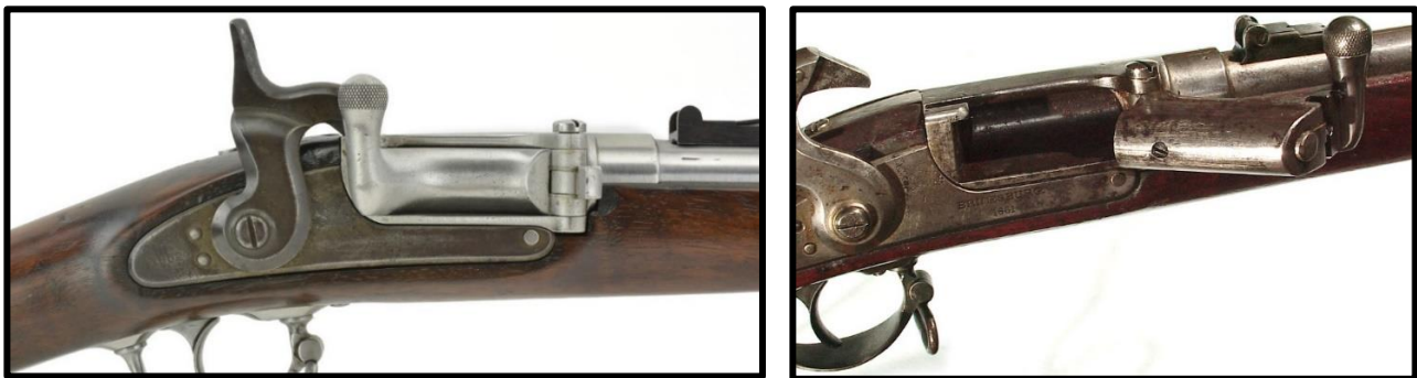
Needham Conversion – close up of closed action at left and open action on right
